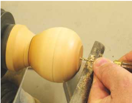
▲ Pic.6 Drill a hole in the top with the 3mm bit; you could use the tailstock but a drill held in a handle and just inserted into the centre point is much quicker
